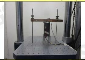
Mechanical Shock Test (-Y axis)
