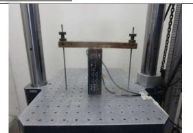
7. Mechanical Shock Test (-X axis)
