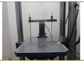
Mechanical Shock Test (+Y axis)
