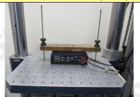
11. Mechanical Shock Test (-Z axis)
