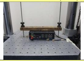
10. Mechanical Shock Test (+Z axis)
